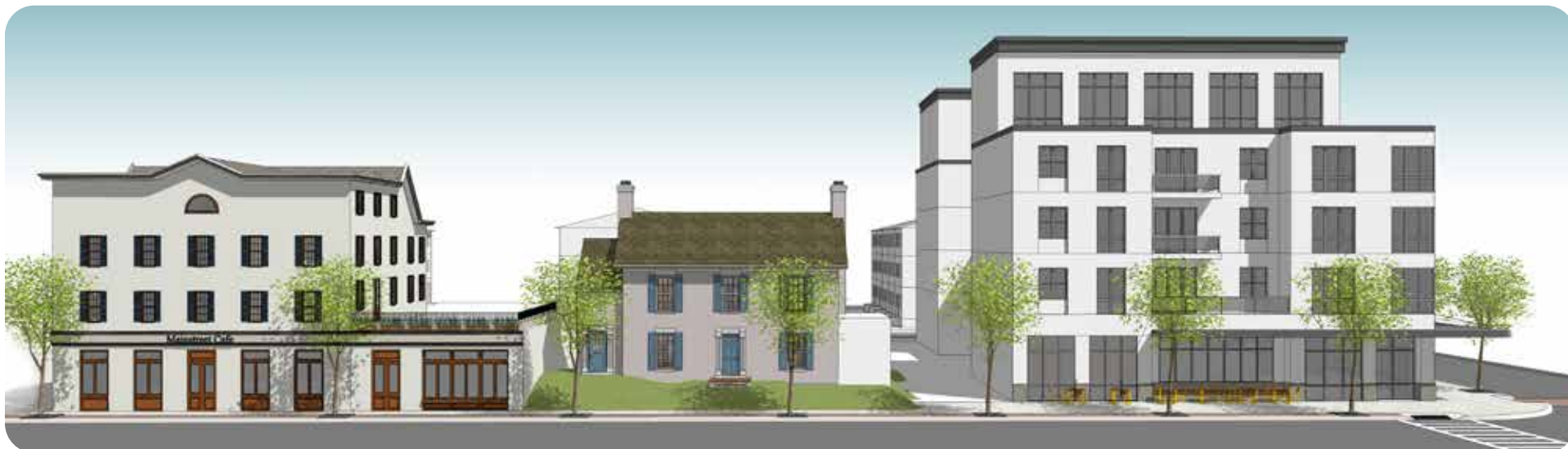
FIGURE 14.5 | EXAMPLE OF FACADE UPGRADES, ADAPTIVE REUSE, AND “STEPPED-BACK” FIFTH STORY IN MIXED-USE CENTER LAND USE
